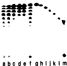
Fig. 4. HPTLC on silica gel. Lanes a–e, time course of oligogalacturonic acid formation resulting from partial hydrolysis of polygalacturonic acid by purified endo -polygalacturonase (0.5, 1, 2, 3 and 4 h, respectively); lane f, oligogalacturonic acid profile resulting from partial hydrolysis of polygalacturonic acid by pectinase; lanes g–m, galacturonic acid, and pure oligogalacturonic acids DP-2 through DP-7, respectively.
